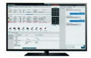
Integrated Text-to-9-1-1 allows users to handle text and voice calls simultaneously. The conversation between the call taker and texter is displayed on the SMS tab on the far right side of the screen.
